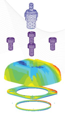
"MSC Nastran reduced the weight by a factor of two, while maintaining the required optical and structural performance"
